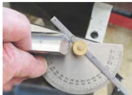
▲ Pic.3 The angle is around 40° although the majority of spindle roughing gouges have an angle higher than that; this takes away the cutting effectiveness of the tool
